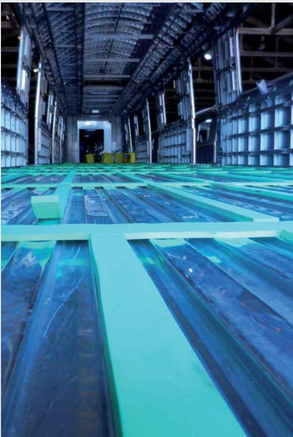
Floating floors for rolling stock
