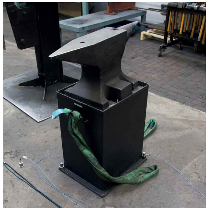
Image 3: Location of acceleration pick-ups in the forge
