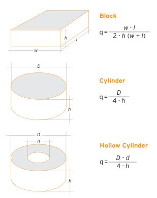
Fig. 4: Definition of the shape factor, block, cylinder, hollow cylinder
