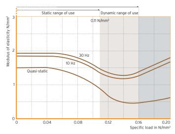
Fig. 3: Load dependence of the quasi-static and dynamic modulus of elasticity, using the example of Sylomer  $\!\circ\!$  SR 110
