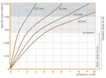
Fig. 2: Load deflection curve, using the example of Sylomer<sub>®</sub> SR 110
