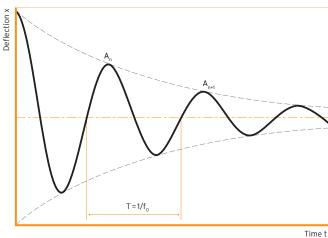
Fig. 8: Fading behavior of a free vibration displacement x
