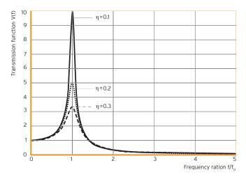
Fig. 9: Transmission function
