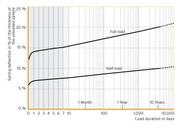
Fig. 5: Static long-term durability of Sylomer®
