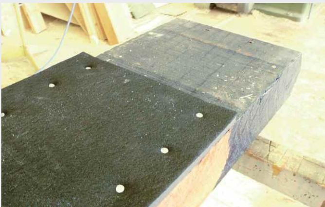
Driving the nails into the material has to be performed very carefully to ensure that the resilient layer is completely attached to the timber sleeper and not penetrated and damaged by the nails.
