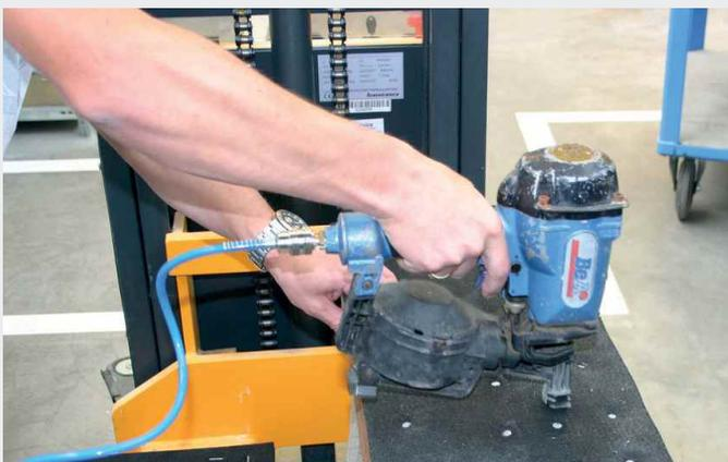
To ensure a proper fixation of the under sleeper pad in the middle of the timber sleeper, at least one additional line of nails should be applied throughout the length of the pad.
