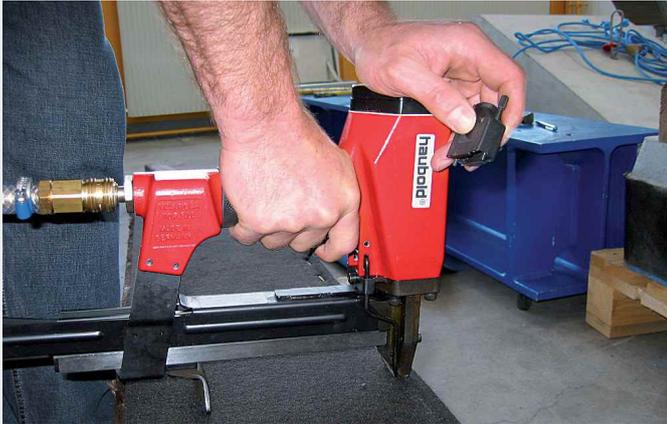
The staples can be applied using a conventional stapling device.
