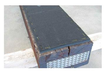
The staples should be placed around the under sleeper pad with a distance of 1 cm to the edge.
