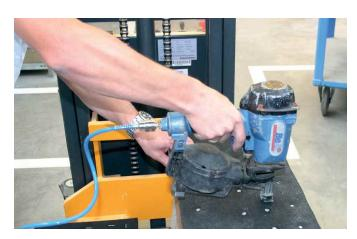
To ensure a proper fixation of the under sleeper pad in the middle of the timber sleeper, at least one additional line of nails should be applied throughout the length of the pad.
