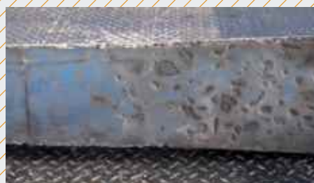
Getzner padding SLB 2210G after 190 million total tons. The plastic impressions in the material prevent shifting by the top ballast layer. No cracks or perforations can be seen in the padding.
