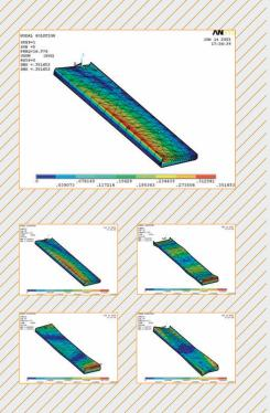
Oscillation forms, calculated using the finite element method (FEM)
