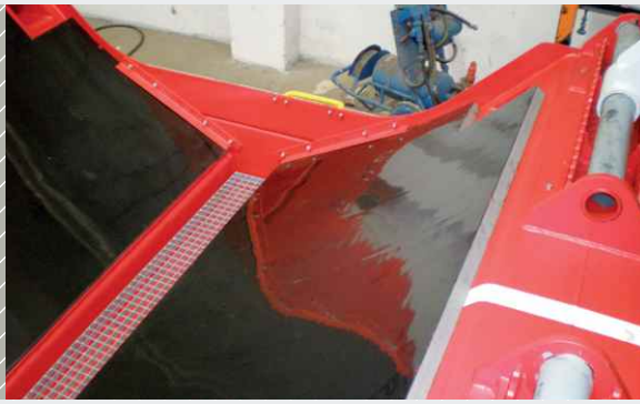
Elastic freight car liner featuring Sylomer®
