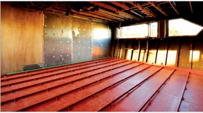
Prepared steel bulkhead
