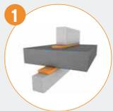
Decoupling of flanking transmission
