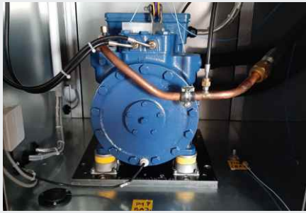
Bearing of a reciprocating compressor with Isotop DZE Mini
