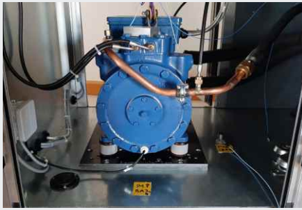
Bearing of a reciprocating compressor with Isotop MSN-DAMP
