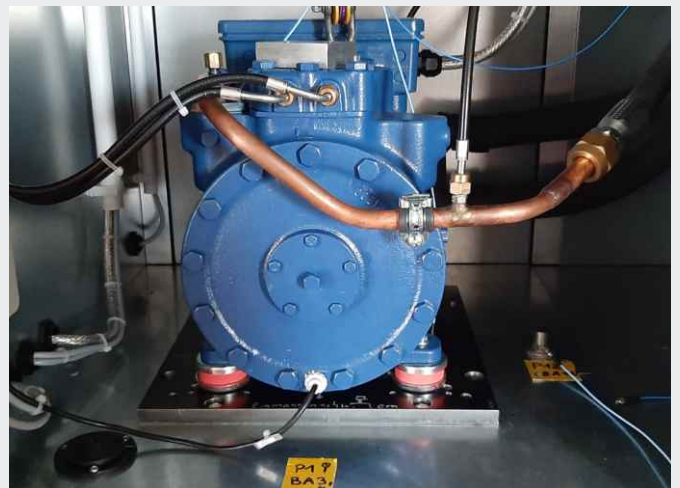
Bearing of a reciprocating compressor with Isotop Compact
