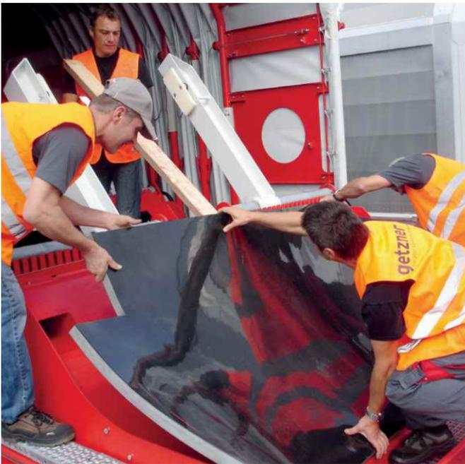
Installation of the elastic freight car liner with Sylomer<sup>®</sup>
