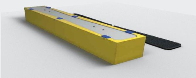
Spacers or centering pins (optional, depending on production method) are placed in order to prevent USP from being completely embedded into the concrete and to keep USP in correct position. It is up to the sleeper manufacturer to ensure proper placement maintaining the correct distances to the outer contour of the sleeper.
