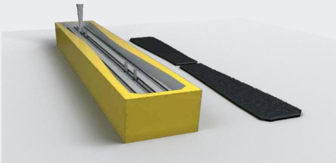
Firstly the sleeper mould is filled with concrete.
