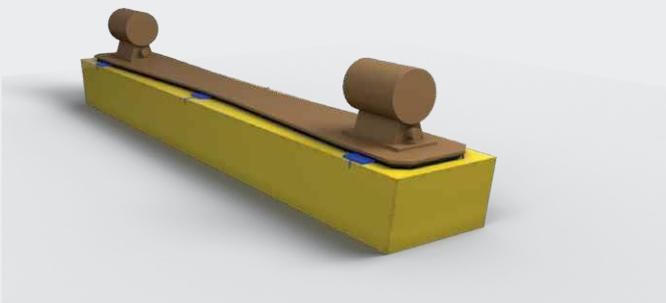
By means of a stiff load distribution plate, covering the whole surface of the pad, the connection layer (mesh or flock) is fully embedded into the fresh concrete. It is recommended to use vibrating motors on the load distribution plate to enable the best connection between USP and sleeper.
