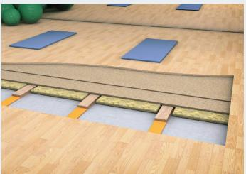
Lots of people moving in time together causes the floor to vibrate. This is especially true when people start jumping in sync or steps are taken in rhythm; these are the kind of vibrations that can be felt in other areas.
