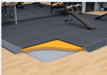
The weight lifting area is often the most critical area in the fitness studio. There is no way to avoid a certain level of impact when it comes to setting down weights and dumbbells. This generates noise and can even damage the floor. Nor do you want weights to bounce back too much because it could cause injuries.
