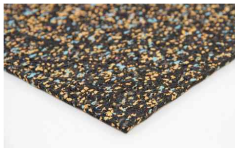
Acoustic Floor Mat 23 Load range: 5000 kg/m 2 Dyn. rigidity s' \leq 35 MN/m 3 Improvement of impact noise \Delta L_{nw} \geq 23 dB
