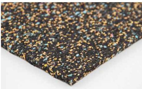
Acoustic Floor Mat 26 Load range: 5000 kg/m 2 Dyn. rigidity s' \leq 20 MN/m 3 Improvement of impact noise \Delta L_{nw} \geq 26 dB
