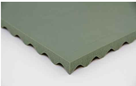
Acoustic Floor Mat 33 Load range: 2500 kg/m 2 Dyn. rigidity s' \leq 13 MN/m 3 Improvement of impact noise \Delta L_{nw} \geq 33 dB
