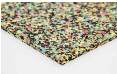
Acoustic Floor Mat 21 Load range: 2500 kg/m 2 Dyn. rigidity s' \leq 40 MN/m 3 Improvement of impact noise \Delta L_{nw} \geq 21 dB
