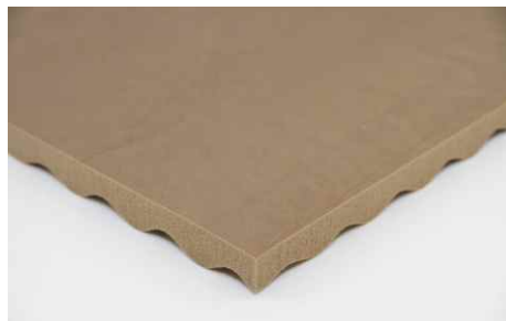
Acoustic Floor Mat 31 Load range: 5000 kg/m 2 Dyn. rigidity s' \leq 17 MN/m 3 Improvement of impact noise \Delta L_{nw} \geq 31 dB
