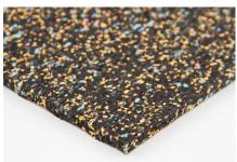
Acoustic Floor Mat 26 Load range:  $5000 \, kg/m^2$ Dyn. rigidity  $s_t' \le 20 \, MN/m^3$ Improvement of impact sound  $\Delta L_w \ge 26 \, dB$
