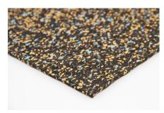
Acoustic Floor Mat 23 Load range:  $5000 \, \text{kg/m}^2$ Dyn. rigidity  $s_t' \leq 35 \, \text{MN/m}^3$ Improvement of impact sound  $\Delta L_w \geq 23 \, \text{dB}$
