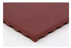
Acoustic Floor Mat 35 Load range:  $2500 \, kg/m^2$ Dyn. rigidity  $s_t' \le 5 \, MN/m^3$ Improvement of impact sound  $\Delta L_w \ge 35 \, dB$
