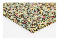
Acoustic Floor Mat 21 Load range:  $2500 \, \text{kg/m}^2$ Dyn. rigidity  $s_t' \leq 40 \, \text{MN/m}^3$ Improvement of impact sound  $\Delta L_w \geq 21 \, \text{dB}$
