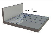
Use a chalk line to create gridlines according to the installation plan on the substrate make for placement of the floor blocks.
