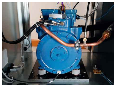
Bearing of a compressor with Isotop® MSN-DAMP
