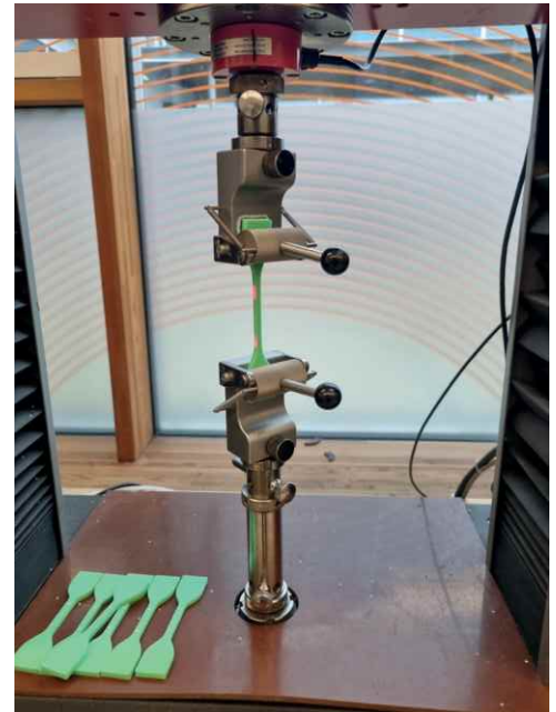
The tensile strength was tested in accordance with DIN ISO 527-1.
