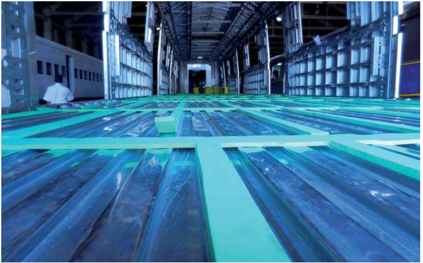
Vibration mitigation with Sylomer® FR floating floors for rolling stock
