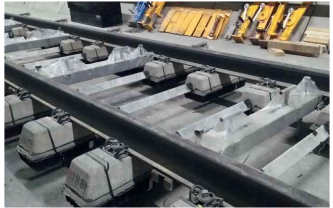
Bi-block sleepers with Syldyn® insertion pads for sleeper boots
