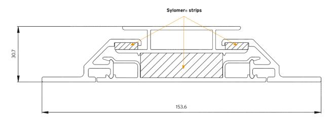
The natural frequencies can be controlled by the profile distances and can therefore be individually adapted. The maximum deflection stated is based on the maximum line load when the maximum permissible weight is reached.
