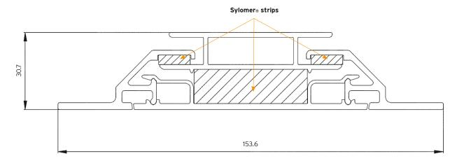
The natural frequencies can be controlled by the profile distances and can therefore be individually adapted. The maximum deflection stated is based on the maximum line load when the maximum permissible weight is reached.
