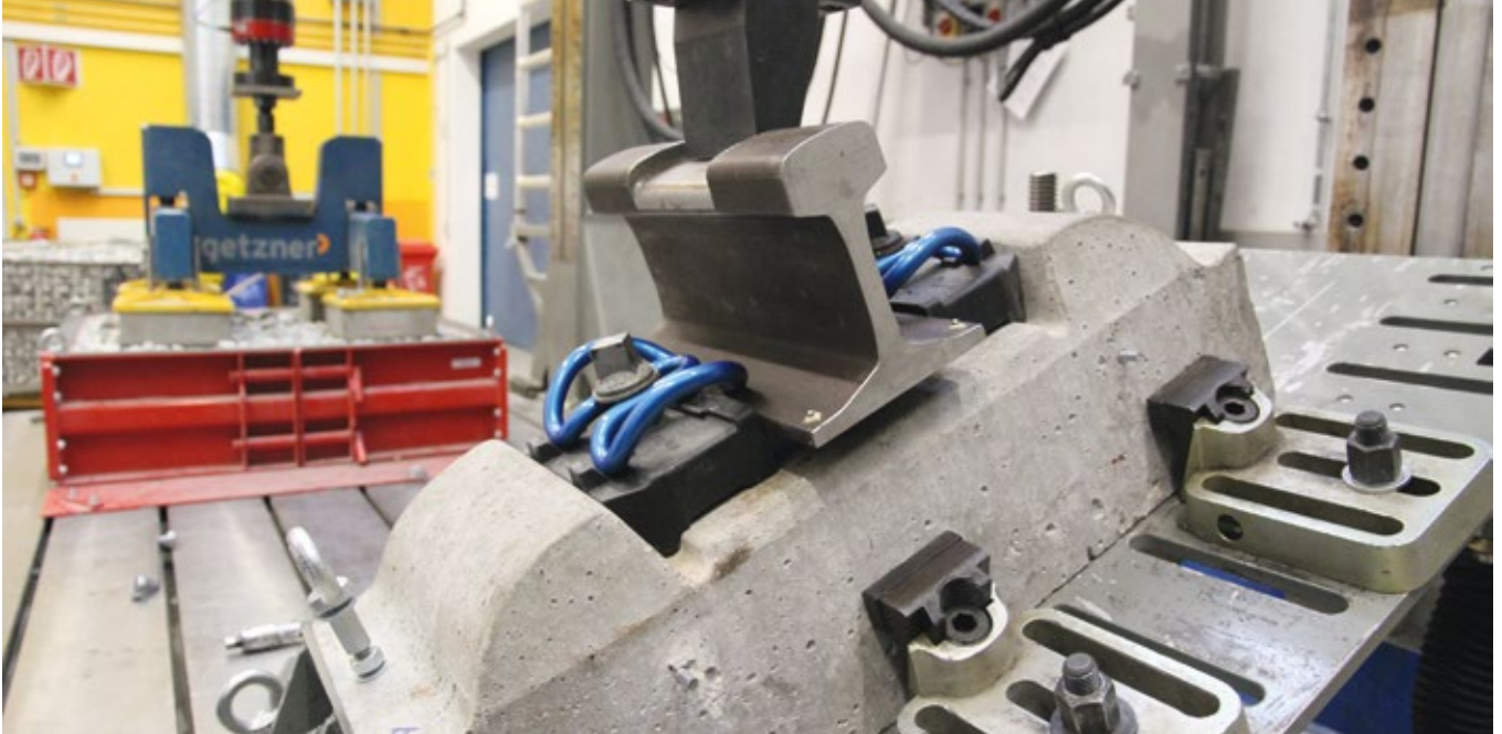
Baseplate pads are subject to intensive testing on the in-house test rig
