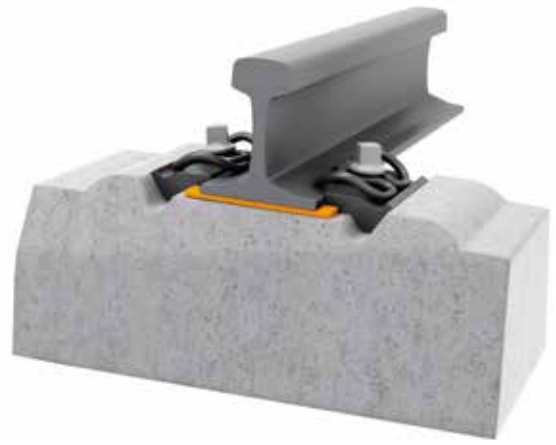
Fig. 1: Left: The railway superstructure emits noise due to vibrating rails and sleepers. Right: Dampening rail pads (orange) placed between rails and sleepers reduce the amplitude of vibrations and, thus, reduce noise.
