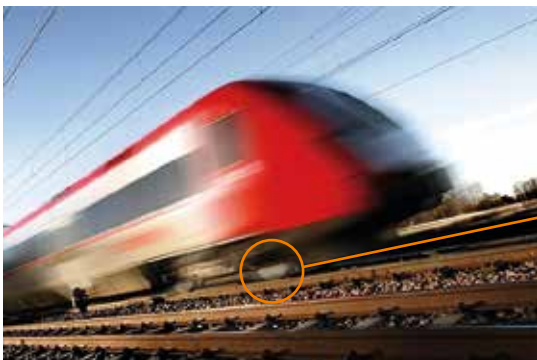
Fig. 11: Noise caused by railway traffic: the interaction between the wheel and the rail causes the wheels, rails and sleepers to vibrate [5], generating airborne noise.
