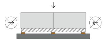
In order to avoid lateral forces, roof units have to be provided with a windbreak.
