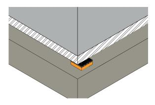
The elements must be positioned completely under the corners of the concrete foundation.
