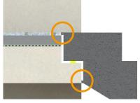
11) Keep elastic joints free of plastering and thick layers of paint to avoid noise bridges!
