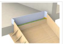
8B) Place the reinforcement of the staircase according to static requirements.
