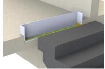
8A) Lift in the prefabricated staircase and place it accurately.Do not damage or remove the bearing.
