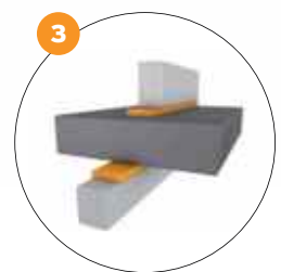
Separation of adjacent components (flanking sound)
