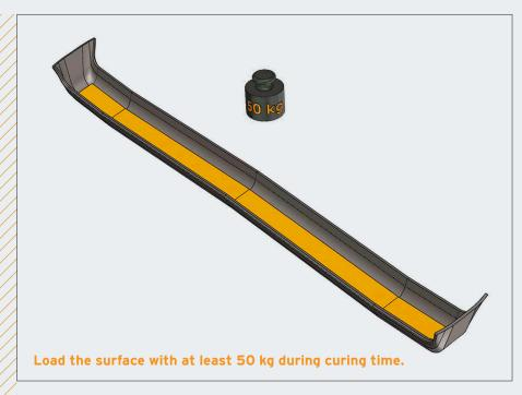
During curing time the pad is even loaded on the whole surface with at least 50 kg or fixed with adhesive tape. After bonding there should be no cavities, which are not filled up with adhesive. The total thickness of adhesive should not be more than 5 mm, because the stiffness of the system could be influenced.
