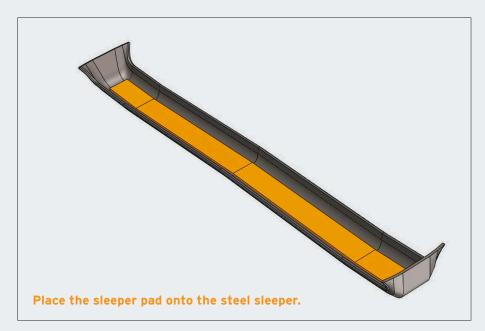
The prepared adhesive is put on the ballast side of the sleeper. If the pad is divided in parts, the joints also have to be bonded. The required amount of adhesive is given by the roughness of the steel surface. Normally per sleeper is used 1/2 to 2 kg adhesive. The coated pad is placed centred on the sleeper.
