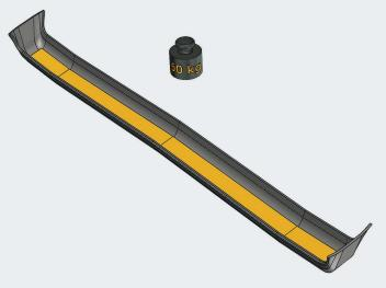
The under sleeper pad is placed centrically on the sleeper. During curing time the pad should be evenly loaded with at least 50 kg. After bonding there should not be any cavities, which are not filled with adhesive. The adhesive layer should be as even as possible (not more than 5 mm thickness difference), in order to avoid any influence on the system stiffness.
