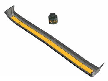
The Under Sleeper Pads are placed centrically on the sleeper. During curing time the pad should be evenly loaded with at least 50 kg. After bonding there should not be any cavities, which are not filled with adhesive. The adhesive layer should be as even as possible (not more than 5 mm thickness difference), in order to avoid any influence on the system stiffness.
