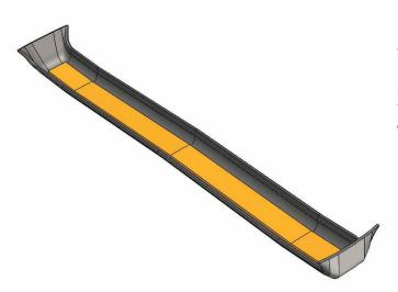
The prepared adhesive is applied on the Under Sleeper Pads. If the pad is divided in parts, the joints also have to be bonded. The required amount of adhesive is given by the roughness of the sleeper surface. Normally 0.5 to 2 kg adhesive is used per sleeper.
