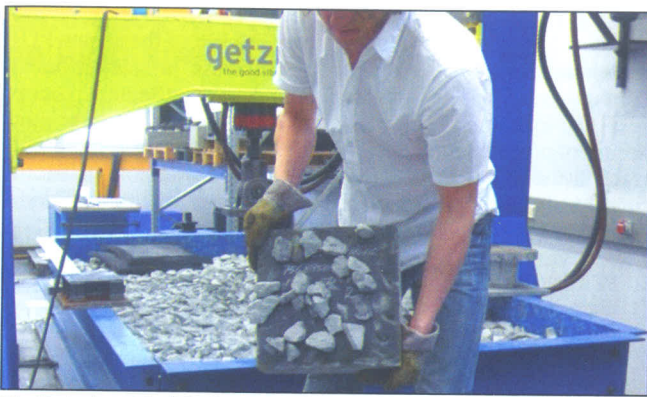
Fig. 5: At the end of the long-term fatigue strength test, the ballast grains remained embedded in the PUR material
