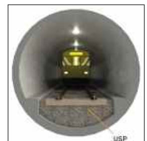
Below: Fig 4. Use of under-sleeper pads in the ballast structure of a single-bore tunnel.
