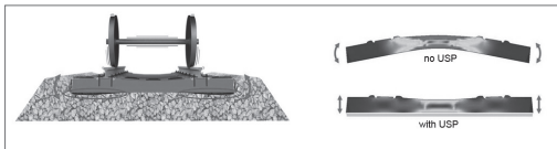
[Figure 3] Void formation only under unpadded concrete sleepers. Such voids are avoided by using under-sleeper pads, which makes load transfer more even
