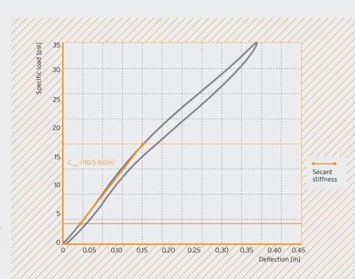
Spring load deflection curve for Sylodyn\_ $_{\otimes}$  DN 335 sub-ballast mat
