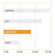
Experimental set-up: 50 kg – 50 cm drop height 18 mm sports floor (16 kg/m²) 25 mm Shock Absorb advanced (5 kg/m²) 140 mm reinforced concrete ceiling (350 kg/m²)
