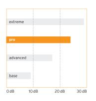
**Experimental set-up:** 50 kg – 50 cm drop height 18 mm sports floor (16 kg/m<sup>2</sup>) 50 mm Shock Absorb pro (10.13 kg/m<sup>2</sup>) 140 mm reinforced concrete ceiling (350 kg/m<sup>2</sup>)
