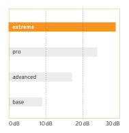
Experimental set-up: 50 kg – 50 cm drop height 18 mm sports floor (16 kg/m²) 75 mm Shock Absorb extreme (22.75 kg/m²) 140 mm reinforced concrete ceiling (350 kg/m²)
