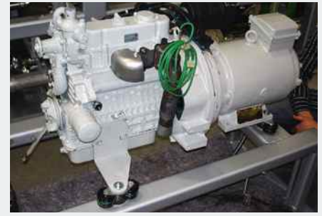
Small combined heat and power plant on Isotop DMSN-BL (special version)
