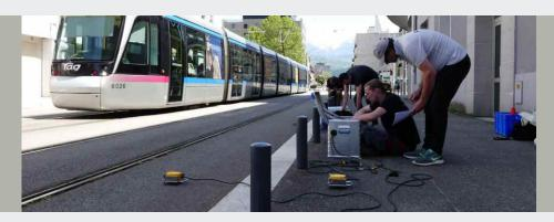
The structure-borne noise insulation was determined by means of 16 measurements using vibration sensors on the on the elastically Sylomer® supported slab and the isolated pavement.
