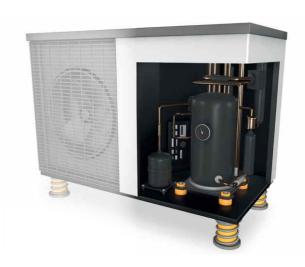
The additional baseplate offers the advantage that bearings can be optimally selected, i.e. so they are closer to maximum capacity and therefore have a lower natural frequency. This is particularly advantageous for lighter scroll compressors in heat pumps or air handling units.
