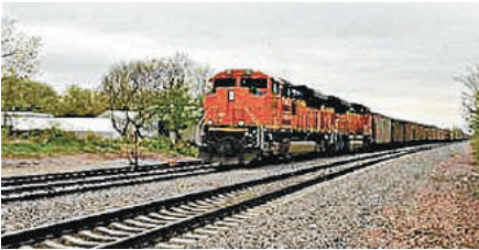
+ FIGURE 4 Thirty-three-tonne-axle-load heavy-haul trains operate on this track section in North America.
