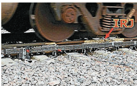
+ FIGURE 5 LEFT Rail deflection was measured at four locations close to the IRJ. RIGHT More uniform rail deflection of padded IRJ (○) versus non-padded IRJ (□) in the immediate IRJ vicinity leads to extended long-term performance.
