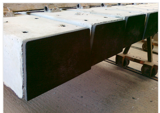
Figure 10: concrete sleeper with USP including a special elastic bearing on both front ends of the sleeper for additional vibration isolation (left: schematic 3D image, right: photograph).
