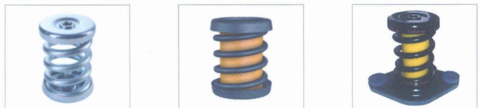
Fig. 3 a) Steel spring; 3 b) Spring with integrated elastomer damper; 3 c) Spring assembly with damper and additional damper for higher-frequency vibrations transmitted via the steel helix
