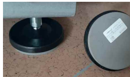
Machine mounting with Sylomer®
